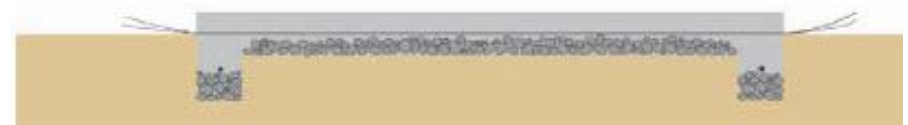
c. A reinforcing grid of tie wire is laid; concrete is troweled in.
